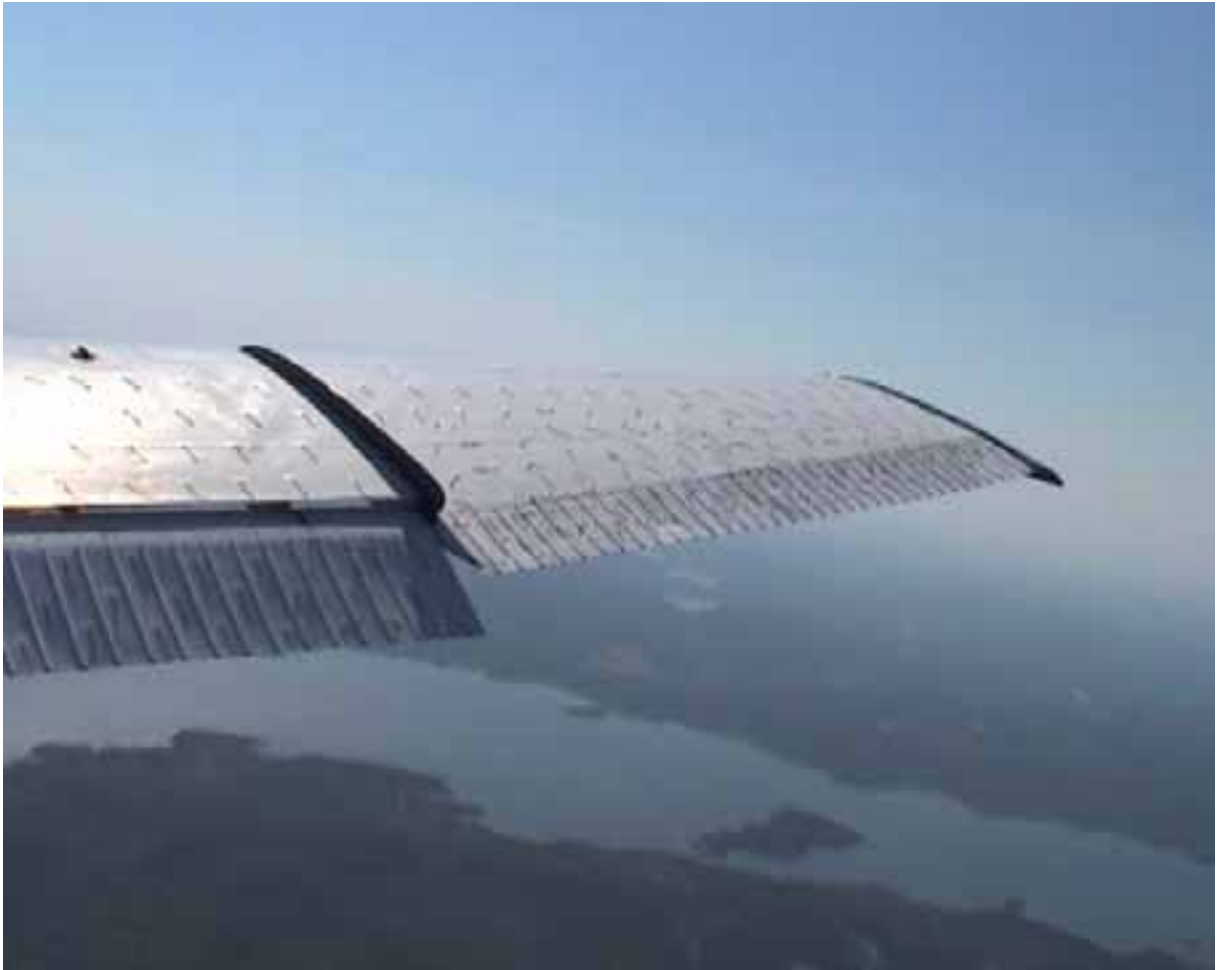
Figure 9. Airflow separation from the right wing tip when stall begins.
