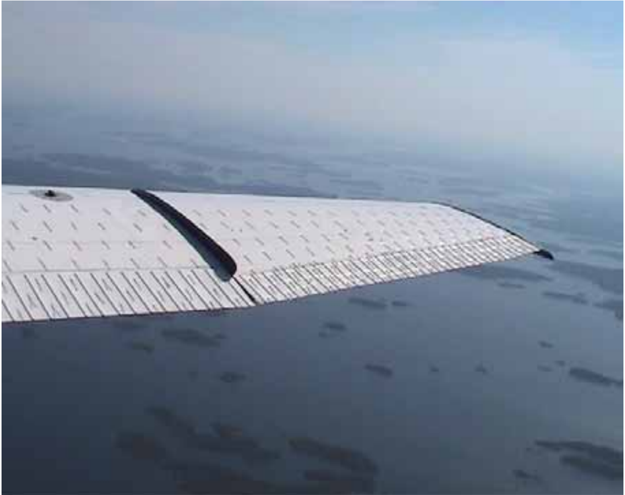
Figure 7. Right wing with flaps up and aileron neutral. The flow is attached to the wing upper surface.
