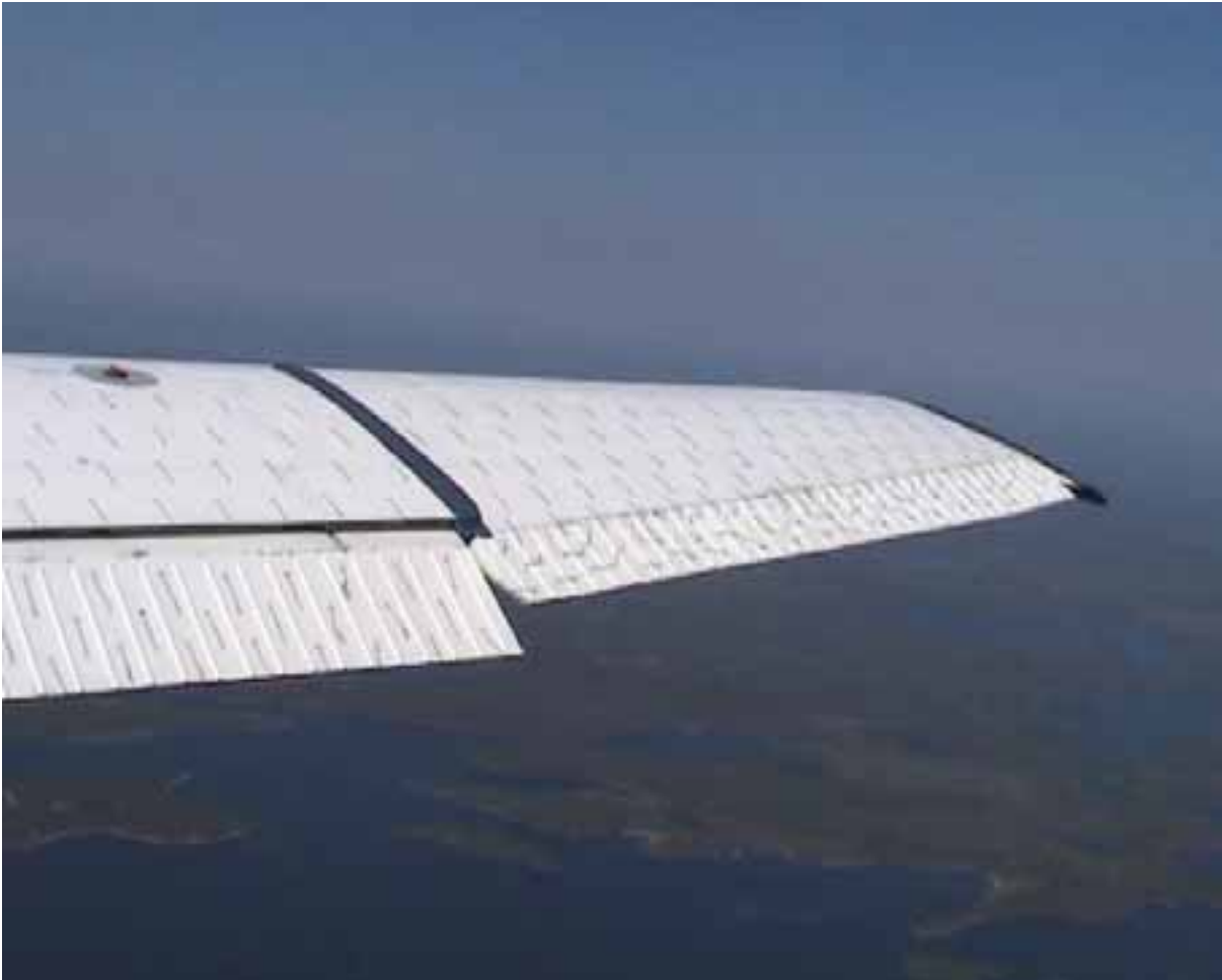
Figure 8. Flap in take off position ( 20^\circ ), when the aileron is at a 13^\circ angle, air speed 80 kt. The flow separation can be seen from the wool threads.
