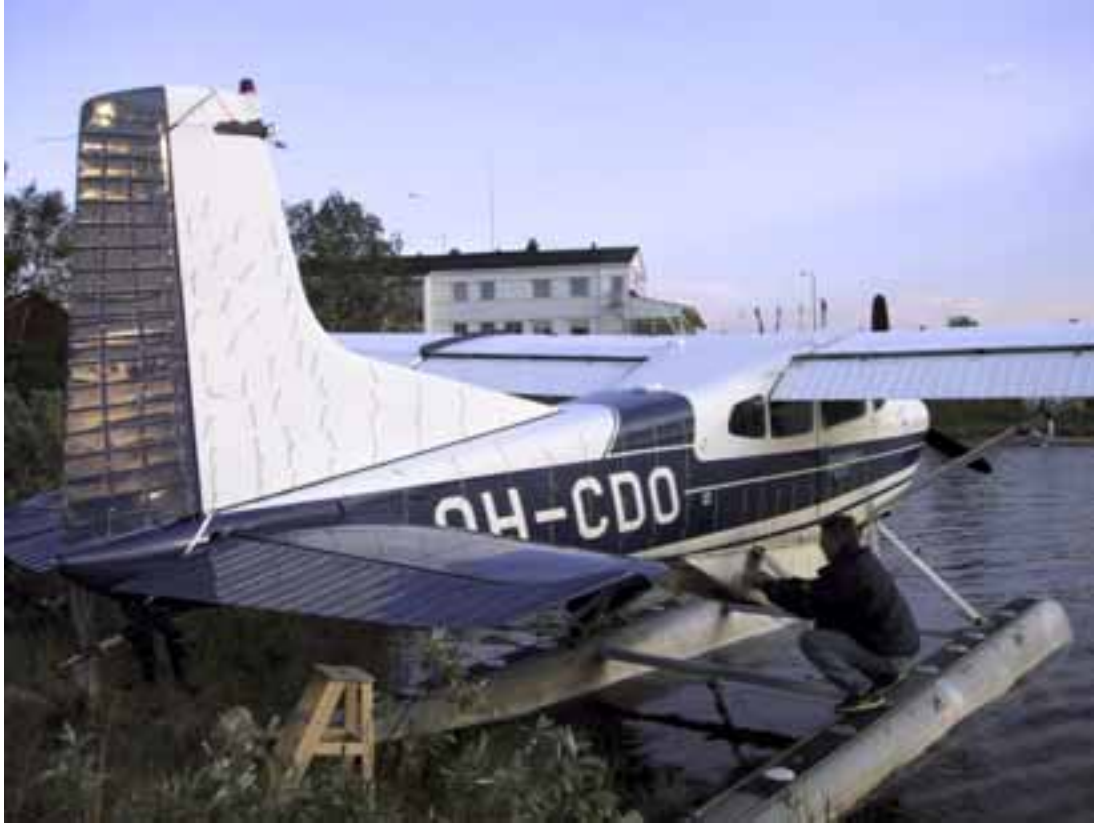
Figure 3. Aircraft fuselage, empennage and right wing upper surface were covered with wool threads for visualization. Five cameras were used to film their movement.
