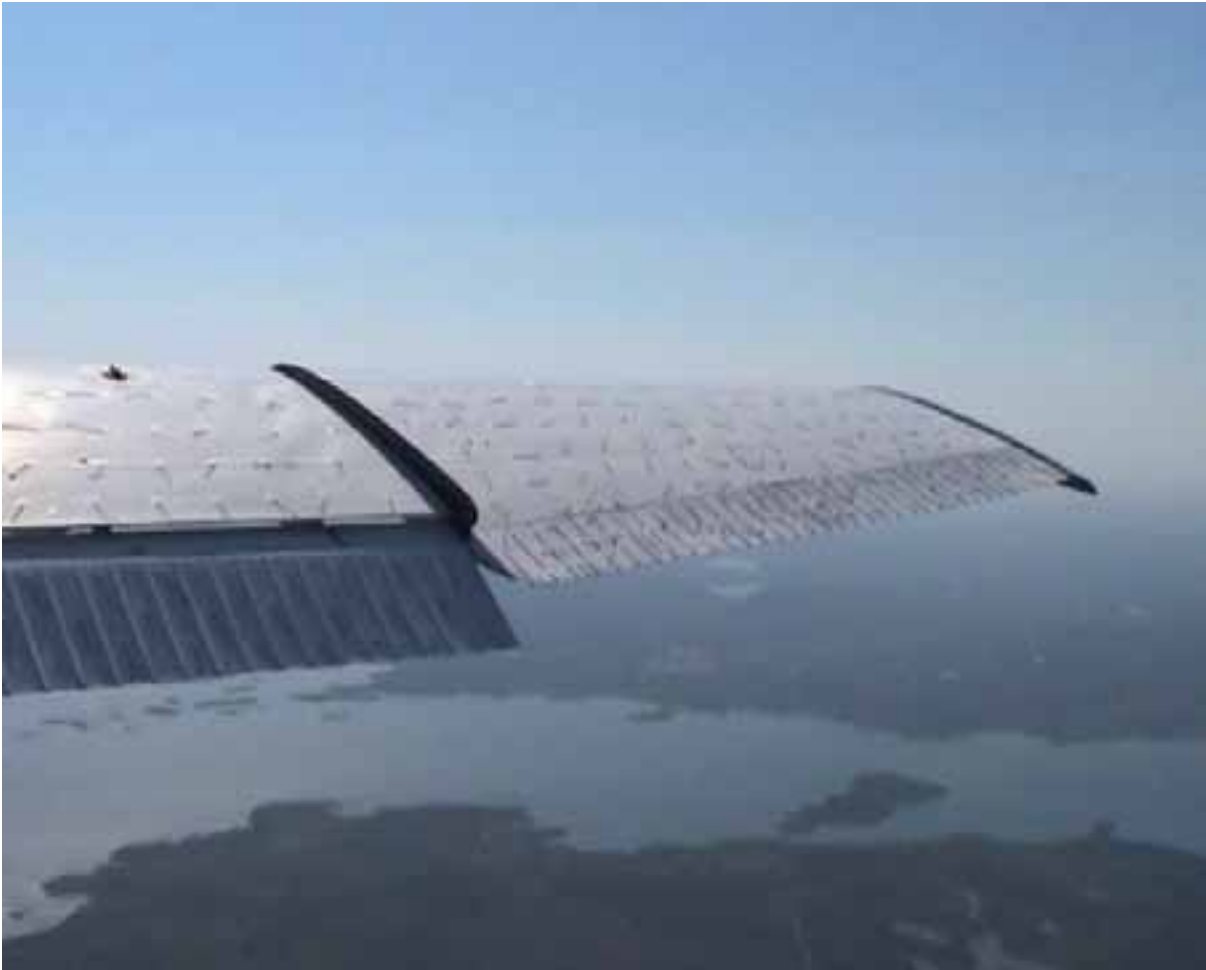
Figure 10. Airflow separation from the whole right wing during a complete stall.
